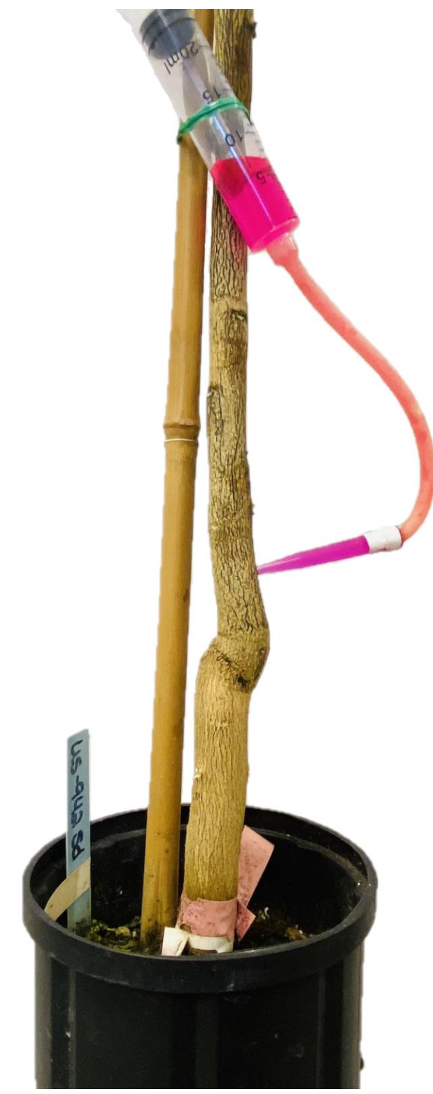
No-pressure injection system : syringe-based device for the direct application of compounds into the xylem.
